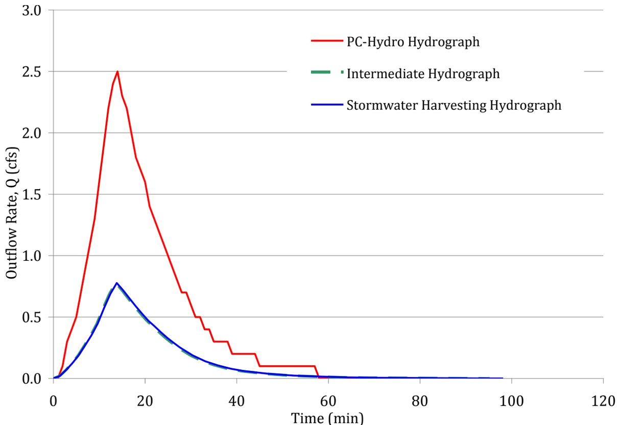
Figure G.3. Stormwater harvesting hydrograph with  $H_{RP} = 0.725$ ,  $\eta_A = 0.95$  and a volume factor = 1.02. The Stormwater Harvesting hydrograph is almost identical to the Intermediate hydrograph in this case.
