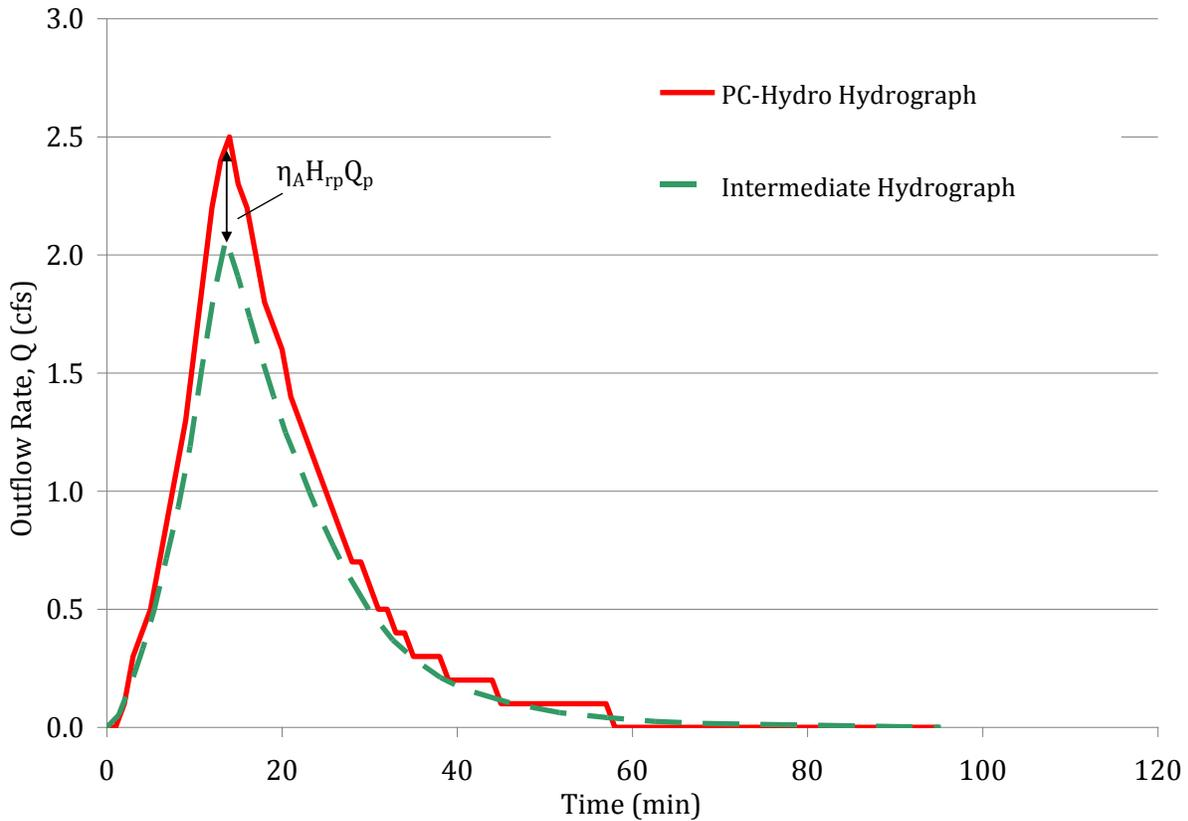
Figure G1. Intermediate hydrograph with peak equal to the reduced peak discharge calculated from Section 3.3.1.
