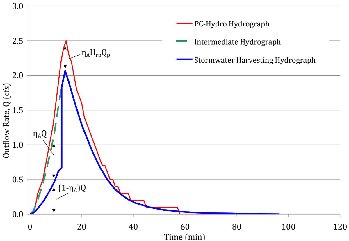
Figure G.2. Stormwater harvesting hydrograph with  $H_{rp} = 0.289$  and  $\eta_A = 0.60$ . The volume factor equals 0.79.
